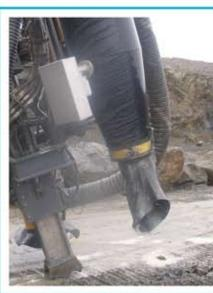
The latest GPS technology (above) is used on our rigs to ensure angled holes are parallel. This is a great advantage especially when working at night or in poor weather conditions where other methods cannot be used accurately.
